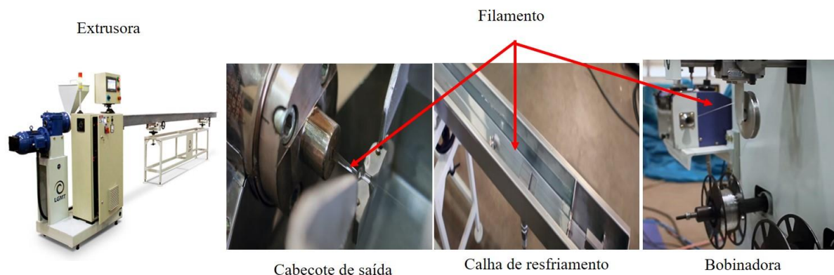
Figure 2 – PLA filament industrial extrusion process
