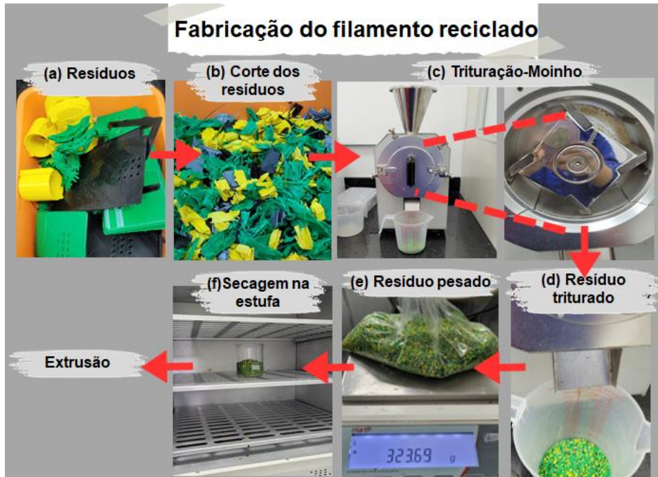
Figure 3 – Manufacturing process of recycled filament (a) Waste. (b) Cutting waste. (c) Grinding in the mill. (d) Crushed waste. (e) Weighing the residue. (f) Oven drying
